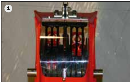
If it doesn't fit, we make it fit: the adjustable drop trunks. Narrow for small seed and wide for large seed.
