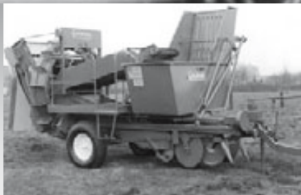
1966: Grimme becomes the market leader with the "Europa Standard" harvester. Share lifting and bunker movement is completely hydraulic.
